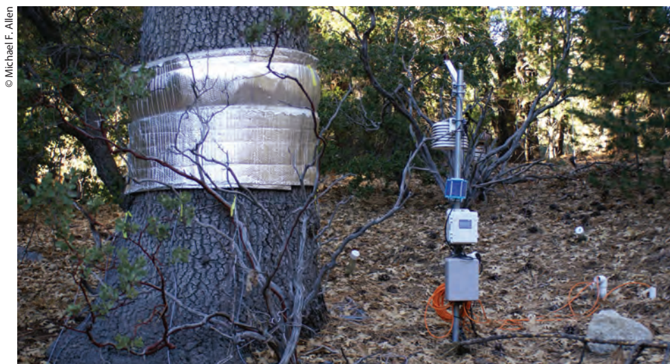
To understand dynamics of black oak interacting with surrounding forest, a thermal-protected sap-flow sensor measures transpiration; a belowground sensor network measures temperature, CO 2 , and soil moisture; and minirhizotrons take images of roots, fungal hyphae, and soil organisms, at the University of California James San Jacinto Mountains Reserve. Hidden nearby is a tower with an eddy flux system measuring CO 2 and water flux between the atmosphere and the canopy, a camera placed on another tower to observe the soil surface, and an eddy flux system to measure flux between the soil surface and the canopy.
